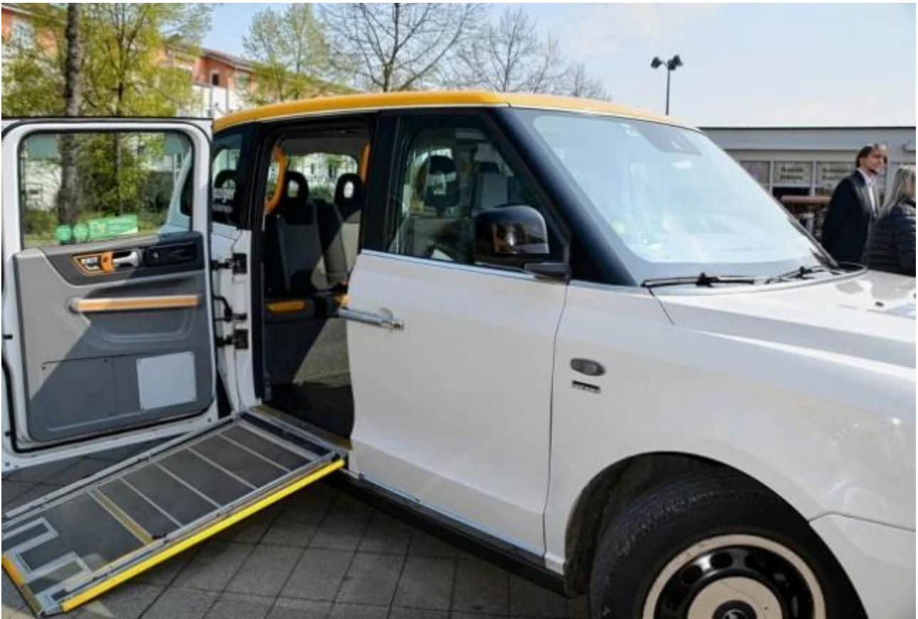
Figure 19: The DRT Flexa vehicles operating in the suburbs of Leipzig have electric vehicles adapted for people with reduced mobility (© Anke Brod)
